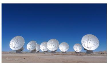
Currently being commissioned at altitude of 5000 m in Chile. Will have 66 telescopes separated by up to 15 kms and observed at wavelength between 7 and 0.35 mm.
